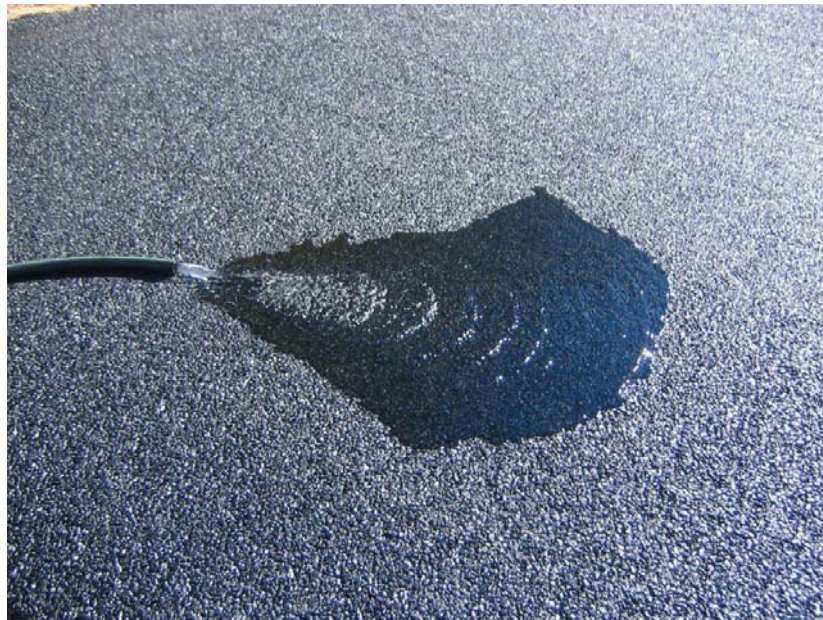
Figure 1. Construction of the UNH porous asphalt lot, October, 2004. Figure 2. Infiltration of 30 gallons per minute from a 2-inch hose at UNH.
