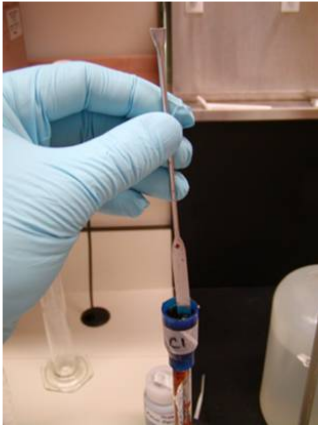
Adding Resin to Column
