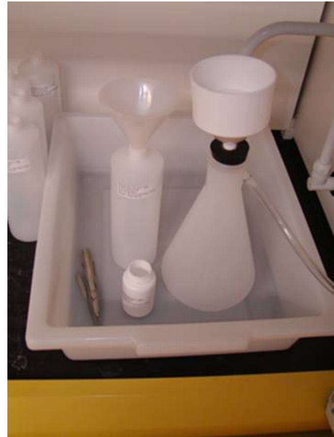
Sample Containers & Filter Setup
