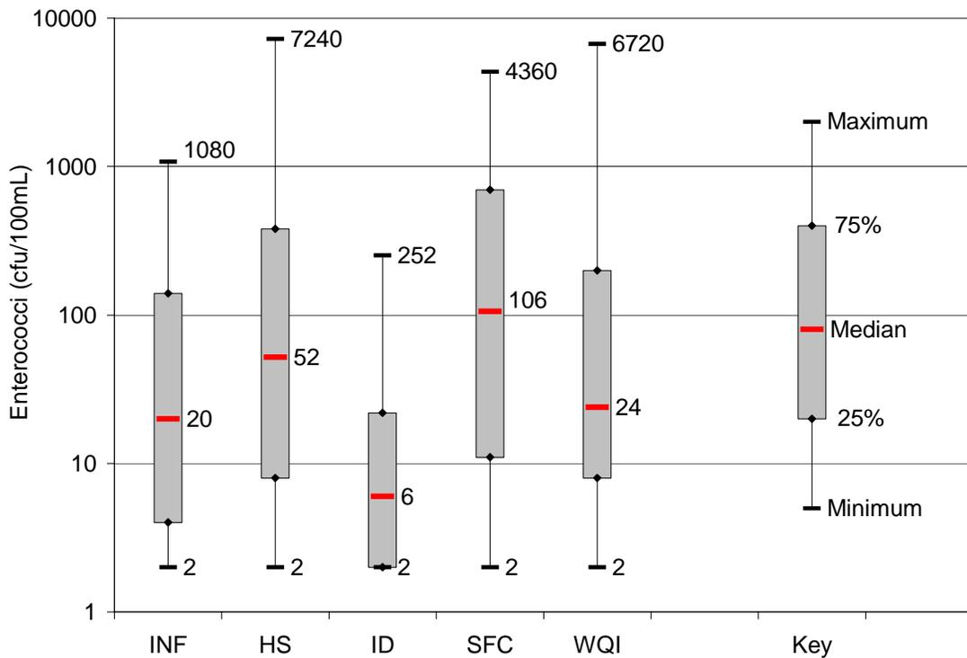
**Figure 4. Variability of dry weather ENT counts by device. Influent (INF), Bioretention Area (BA), Gravel Wetland (GW), Hydrodynamic Separators (HS), Infiltration Drainfield (ID), Rock-lined Swale (RLS), Sand Filter (SF), Stormwater Filtration Chamber (SFC), Wet Detention Pond (WDP), Water Quality Inlet (WQI)**
