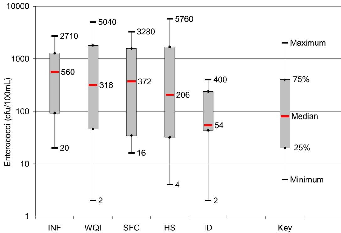
**Figure 2. Variability of storm event ENT counts by device. Influent (INF), Bioretention Area (BA), Gravel Wetland (GW), Hydrodynamic Separators (HS), Infiltration Drainfield (ID), Rock-lined Swale (RLS), Sand Filter (SF), Stormwater Filtration Chamber (SFC), Wet Detention Pond (WDP), Water Quality Inlet (WQI)**
