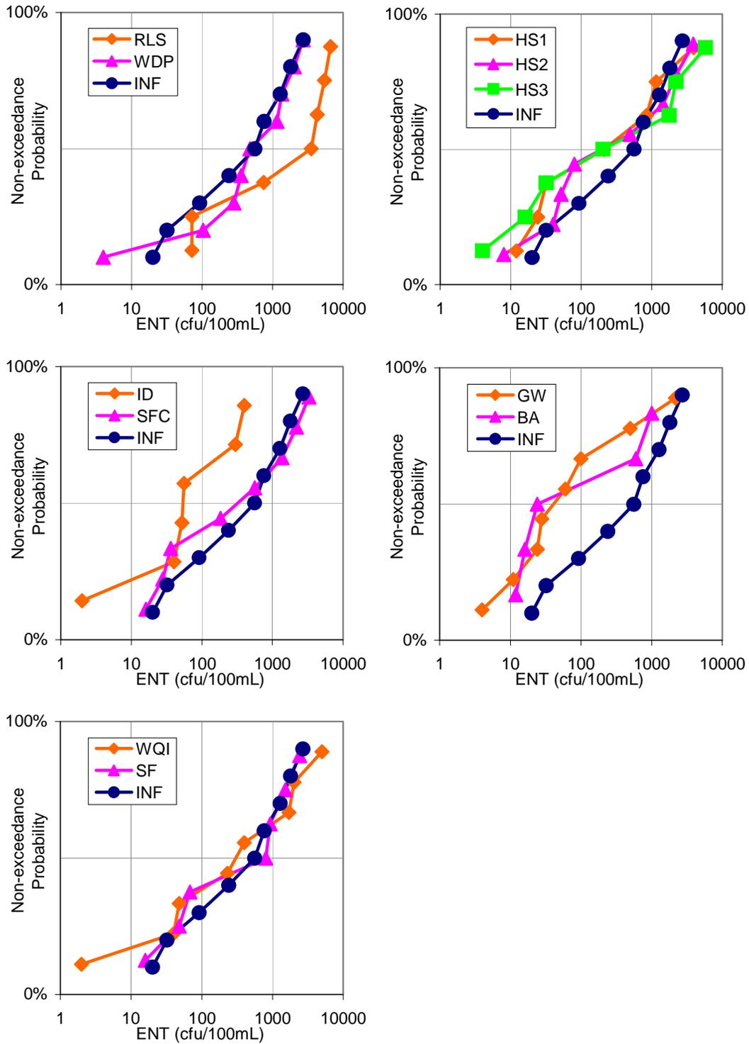
**Figure 3. Non-exceedance Probability Plots For ENT concentrations in Device Influent and Effluent**
