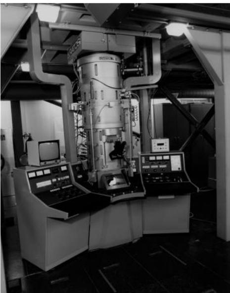
**AEI/Kratos 1 MV transmission electron microscope console.**
