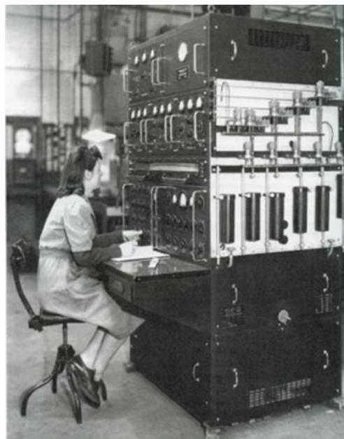
**MS1 (1946): Analysis of isotope ratios in uranium hexafluoride (UF<sub>6</sub>) contained in gas cylinders on the side of the instrument by mathematician Anne Mettrick from MV. This is likely to be the fourth MS1 which remained at MV and was used to develop MS2.**
