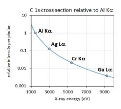
minutes with Al K $\alpha$  X-rays will have to be significantly longer. However, the increase in collection time can be mitigated somewhat by acquiring regions with higher pass energy to increase the sensitivity. It is also noted that for elements Aluminium to Chlorine, the 1s core level and associated KLL Auger electron peak appear as strong features in the Ag L $\alpha$  excited spectrum.
