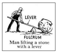
Makes lifting weight easier by using a fulcrum to redirect force over a longer distance. **Examples:** see-saw, dump truck, broom, crane arm, hammer claw, crowbar, fishing pole, screwdriver, bottle opener
