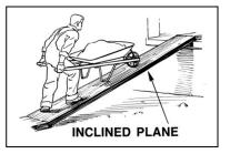
Makes it easier to move objects upward, but you have to go further horizontally. **Examples:** highway or sidewalk ramp, wheelchair ramp, stairs, playground slides
