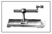
Turns rotation into lengthwise movementTakes many twists to go a short distanceHolds things together
