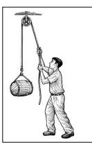
Makes lifting things with a rope easier by redirecting force and the addition of additional pulleys. **Examples:** flagpole, elevator, sails, fishing nets, clothes lines, cranes, window shades and blinds
