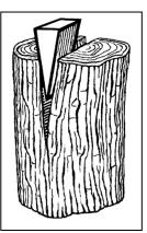
Pushes materials apart, cuts things **Examples:** scissors, knife, doorstop, nail, saw, bulldozer, snow plow, zipper, airplane wing, bow of a boat or ship
