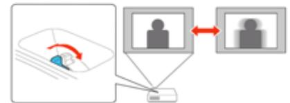
Step 5: If the height of the left and right borders of the projection image are not equal, adjust the slider (next to focus/zoom rings) until equal.
