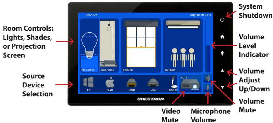
**To adjust system volume**, first raise the volume of the video or audio file, then the device system volume, then the AV touch panel volume buttons. Ensure **Volume Mute** is not enabled. Adjust the classroom environment using the lights, screen, and shade controls on the AV touch panel.
