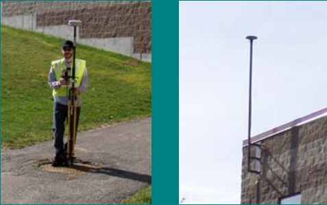
Photo 1 and 2: RTK GPS and UNH Base Station
