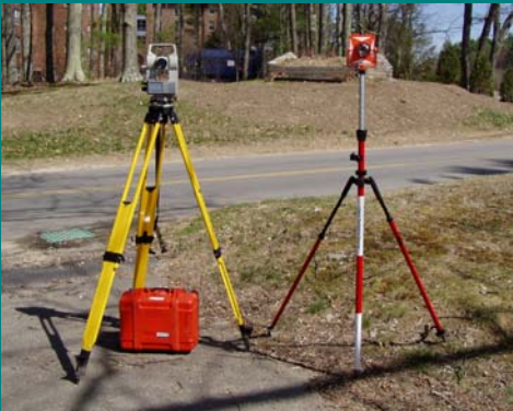
Photo 3: Total Station and Reflecting Rod
