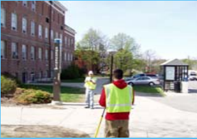
In the field, collecting a point using the offset feature in the RTK unit through the aid of the disto laser measurement tool.
