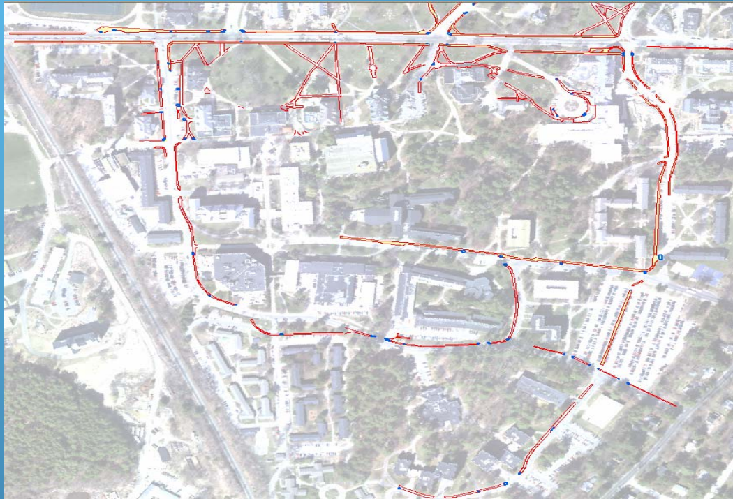
Aerial imagery of UNH Campus used as reference for post processing data in ArcMap software. Figure includes walkways and accessible curb ramps in shapefile and geodatabase feature class formats mapped in the campus' main core area.
