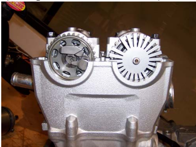
Trigger Wheel Mounted to Cam Shaft
