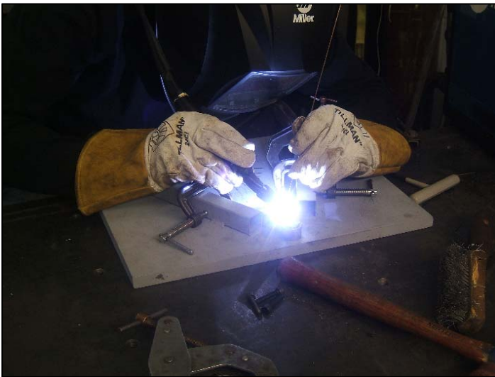
A Team Member Uses a jig to Fabricate Suspension Components
