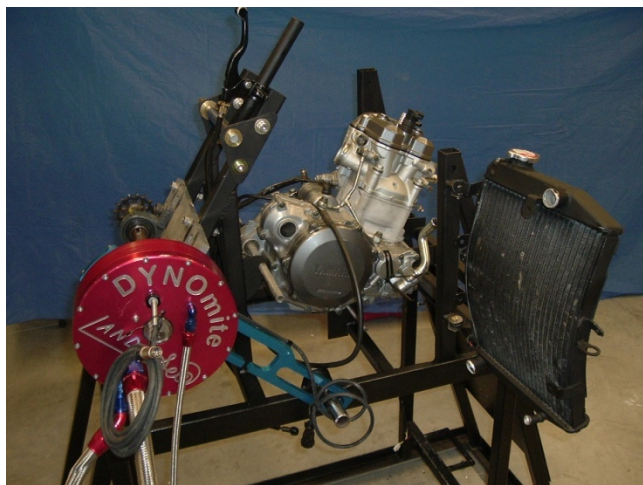
Our YZ450 Engine on the dyno stand
