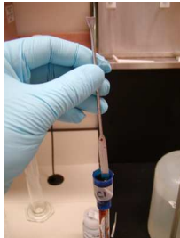
Adding Resin to Column
