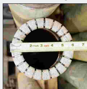
Triple core barrel resulting in 100 mm rock cores.
