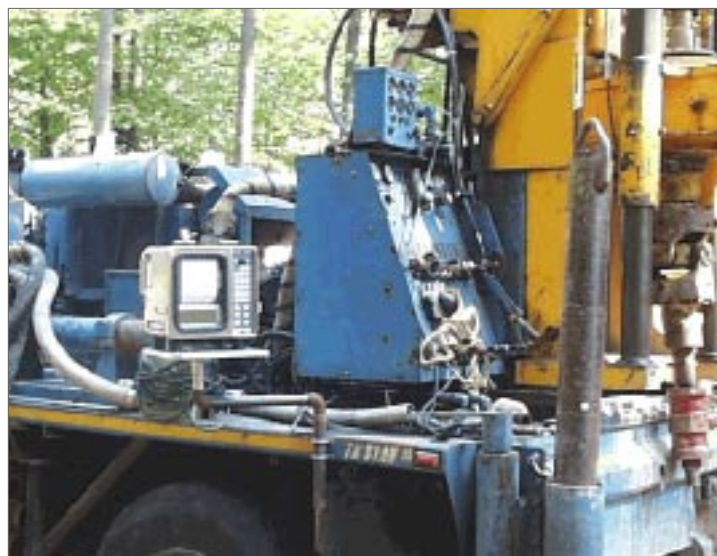
Drilling parameter recorder mounted on a drill rig.
