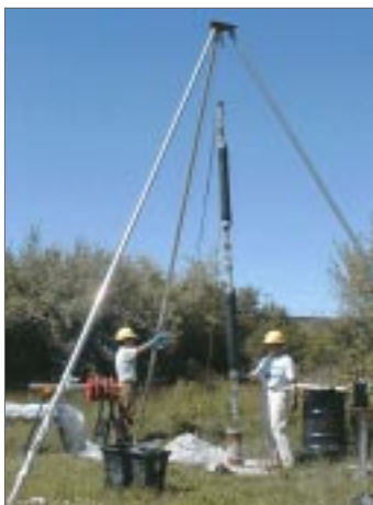
Straddle-packer system used for BBC hydraulic testing.
