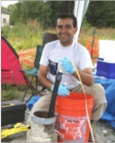
UNH graduate student Gonzalo Pulido-Silva removes diffusion bag samplers from a BBC borehole.
