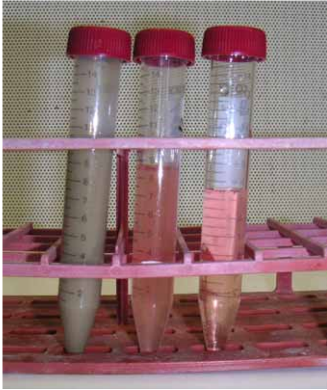
Figure 2. Bacillus atrophaeus spores in phosphate buffered saline. 10^{11} spores/mL, 10^9 spores/mL 10^7 spores/mL (left to right)
