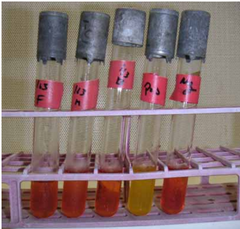
Figure 3. Bacillus atrophaeus spores ( \sim 10^6 spores/mL) after autoclaving. Rudman Hall, Room 163 – Front, Middle, Back, Positive Control, Negative Control (left to right)
