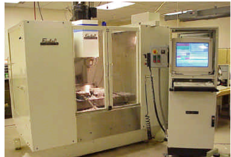
MDSI Open Architecture Controller retrofit on a FADAL VMC Design and Manufacturing Lab - University of New Hampshire
